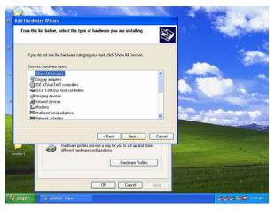
Figure 3.23: Select "Show all devices" in Common hardware types windows
